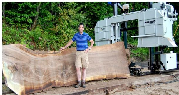
this mill features a saw head with a massive throat opening that moves along a twin-rail frame.
